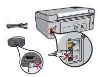
IMPORTANT: If your printer has a USB port on the front, do not attach the print adapter to it. Use the back USB port.
